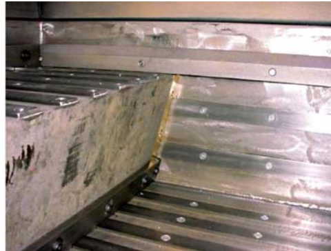
WEIMA hydraulic ram with ram comb plate WEIMA hydraulic ram without ram comb plate
