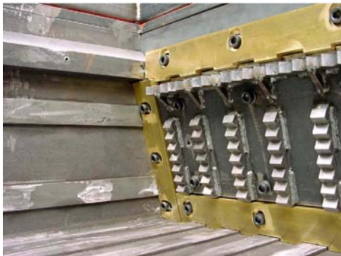
WEIMA hydraulic ram with ram comb plate WEIMA hydraulic ram without ram comb plate
