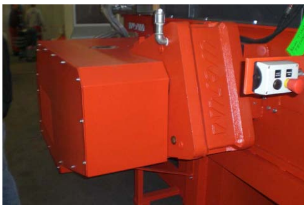
The WEIMA WAP Gearbox – Standard on WEIMA-shredders with an output of 55kW or bigger
