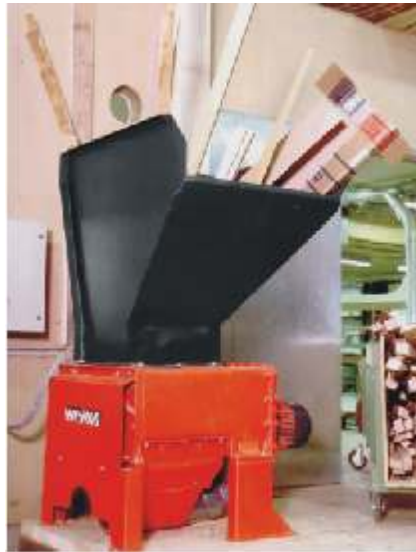
In use in a joiner's shop: 4-shaft shredder of the ZM 30 series with loaded funnel
